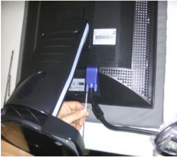
1. At first, remove signal cable with manual driver. (Auto driver can damage plastic screw hole)
