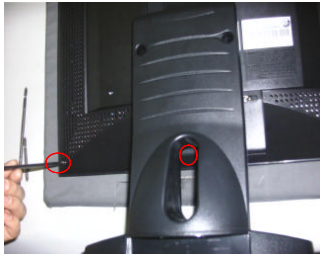
2. Remove back cover screw bolt (5 point) - 4 corner and center of bottom
